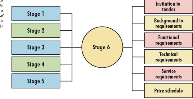
Fig.5.3 The process for compiling a statement of requirements (SOR)
