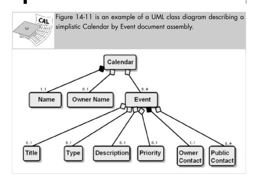
Figure 14-11. Calendar by Event Assembly Model as a UML Class Diagram
