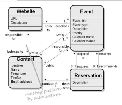
Figure 13-10. Contact Pattern to Consolidate Repeated Structures
